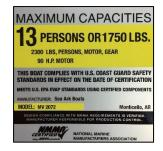
for loading the boats, which are enforceable by law. Never exceed the "U.S. Coast Guard Maximum Capacities" indicated on the capacity plate.
