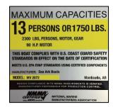
for loading the boats, which are enforceable by law. Never exceed the "U.S. Coast Guard Maximum Capacities" indicated on the capacity plate.
